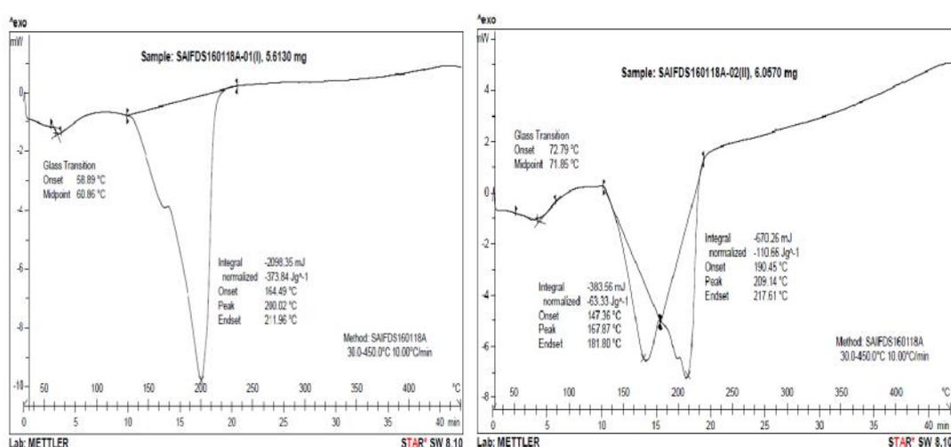
Fig.3. DSC curve of sample type 1 (calcium phosphate) and sample type 2 (calcium oxalate hydrate)
