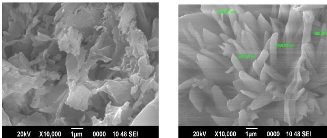
Fig. 4 Scanning electron micrographs of (a) Sample type 1 (calcium phosphate) and sample type 2 (calcium oxalate hydrate)
